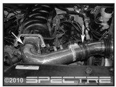
Step 18 Install the long intake tube into the throttle body coupler and then slide the 3.5" coupler back over from the short tube. Once tubes and couplers are in position, securely fasten all clamps.
