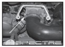
Step 4 Loosen the hose clamp at the throttle body.
