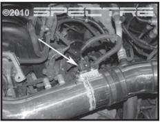
Step 19 **Connect the MAF sensor** connector by pushing the connector on the sensor.
