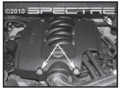
Step 22 Install the engine cover and reinstall the two factory screws
