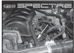
Step 20 Install short breather hose onto driver side valve cover where factory hose was removed from step 8. Connect to intake tube.
